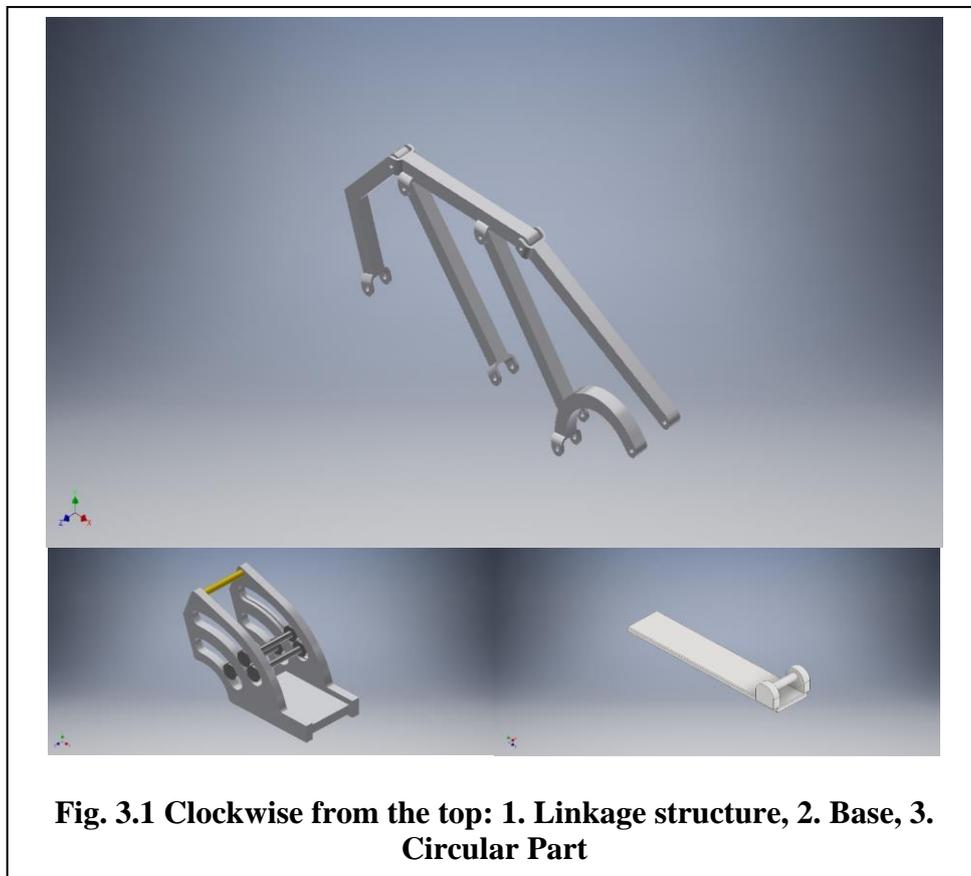
**Fig. 3.1** Clockwise from the top: 1. Linkage structure, 2. Base, 3. Circular Part
